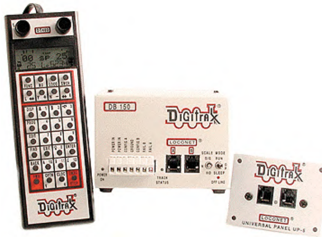
The Empire Builder II Set from Digitrax, DT400, DB 150, and the UP5 (from left to right)
